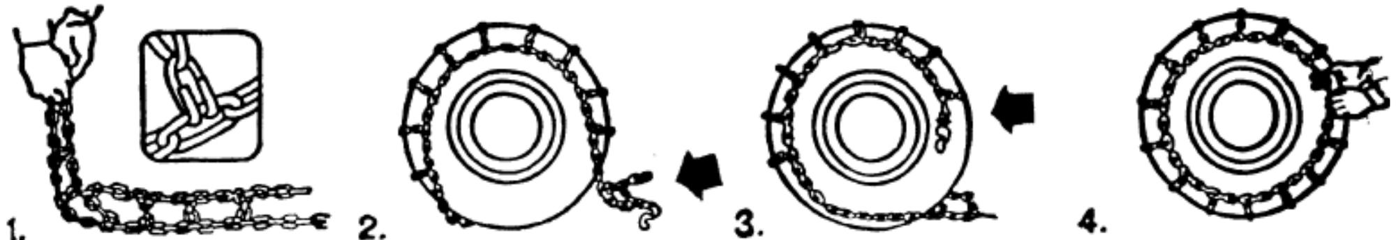
1. Lay chains out flat, remove all tangles. When chains are placed on the tyre, the cross hook eyes must face up (see the insert). Damage to your tyres could result if these hooks face against the tyre.
